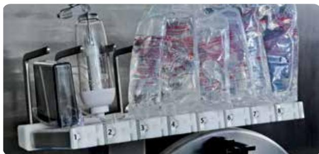
**Syringes, final containers, and drug vials from different manufacturers can be used simultaneously.**
